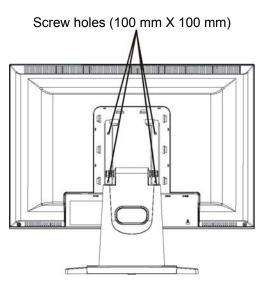
\* Note: Please use UL Listed wall mount bracket with M4 mm x 12 mm (L) screw for application.
